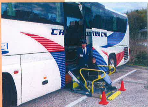
Lift in operation
